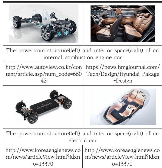
Fig. 1. A comparison of changes in interior space as a result of changes in structure between existing internal combustion engine cars and electric cars
