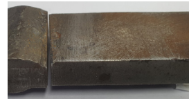
Fig. 11. Specimen cut by wire electrical discharge machining.
