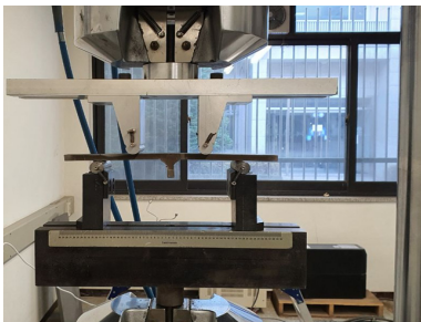
Fig. 15. Fatigue test of fillet weld specimens
