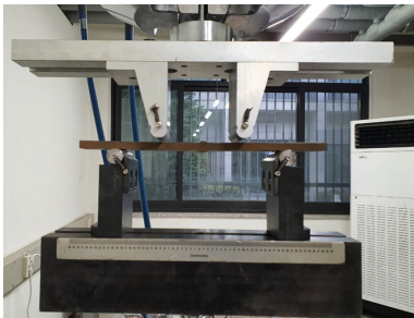
Fig. 14. Fatigue test of butt weld specimens
