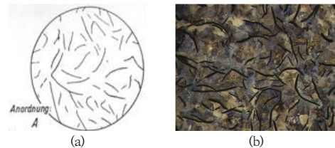
Fig. 8. Microstructure of casting material (a) Reference (b) Localization casting material
