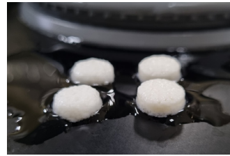
Fig. 4. Macroscopic picture of SR-3(left) and SR-4(right) at 270 minute during dissolution test. SR-4 tablet maintained the initial shape for 4.5 h, but SR-3 tablet was surface-eroded at 4.5 h.
