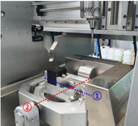
Fig. 2. Photograph of the dental-crown machine with dry machining module.
