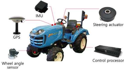
Fig. 2. 20kW Tractor and Component
