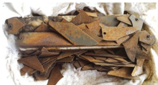
Fig. 2. A failure of the leaf spring caused by corrosion
