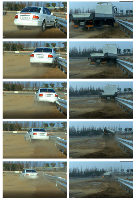
Fig. 4. Sequential photographs of car & truck impact test
