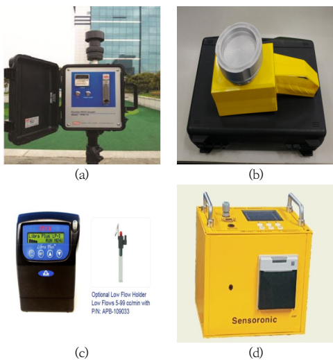
Fig. 3. Measuring Equipment of Indoor Air Quality (a) BMW-3500 (b) SAS HiVAC (c) LP-1 (d) GSR-310
