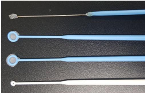
Fig. 2. Temporal vitrification device was produced with nylon mesh and inoculation loop.
