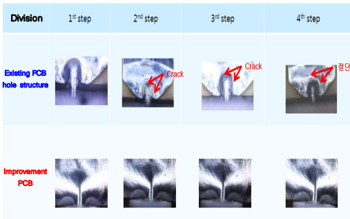
Fig. 17. Fastening structure durability test result
