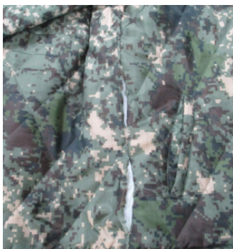
Fig. 2. Side line seam bursting of military winter inner clothing
