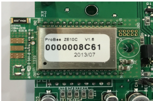
Fig. 7. Zigbee communication unit of automatic recording system for discharge of the wastewater discharge facilities
