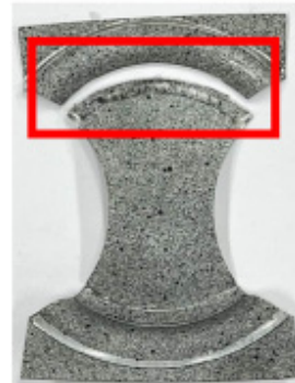
Fig. 10. Fracture at grip area by upper die
