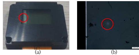
Fig. 7. Photograph of LCD liquid crystal failure (a) LCD panel (b) Damage area of liquid crystal
