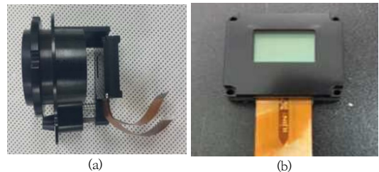
Fig. 2. Photograph of Ocular and LCD panel (a) Ocular (b) LCD panel
