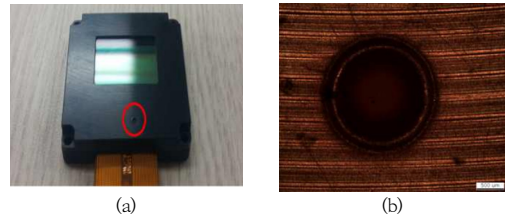
Fig. 6. Photograph of LCD panel housing failure (a) LCD Panel (b) Damage area of housing
