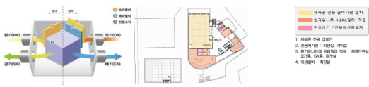
Fig. 5. Ventilation unit (HEPA filter) / Planning of Ventilation Facilities on 3F of Jiphyeon-dong Complex Community Center [2]
