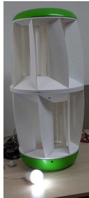
Fig. 5. Final product of dual small wind generator
