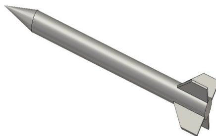
Fig. 11. Represents the missile with the dimensions 580 mm x 120 mm x 120 mm
