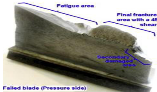
Fig. 8. Blade(Pressure side) damaged
