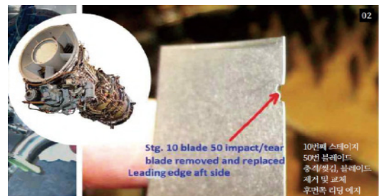
Fig. 1. FOD Damaged Compressor Blade
