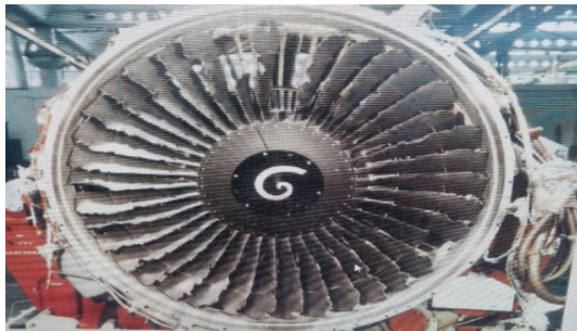
Fig. 6. Damaged blades by flutter in gas turbine
