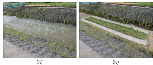
Fig. 12. Hydraulic stability test(2nd, vegetation) (a) before, (b) after
