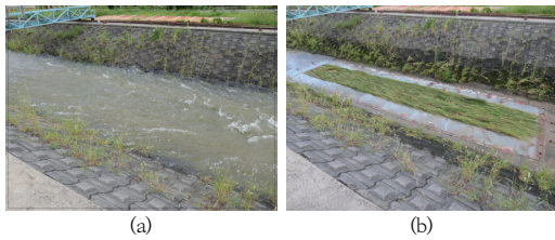
Fig. 13. Hydraulic stability test(3rd, vegetation) (a) before, (b) after
