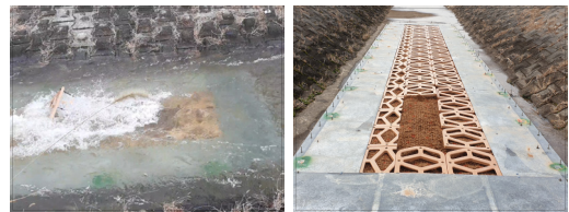
Fig. 10. Hydraulic stability test(2nd, no vegetation)
