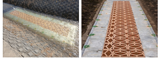
Fig. 9. Hydraulic stability test(1st, no vegetation)
