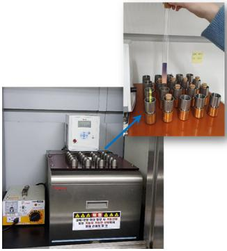
Fig. 2. Equipment for heat stability test
