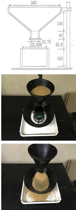
Fig. 1. Main specifications of bulk density measuring device (mm) and bulk density measuring device
