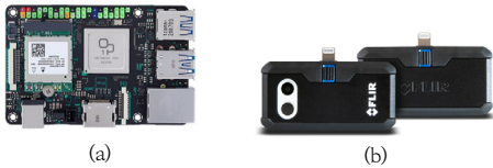
Fig. 2. Thermal Imaging Camera Part (a) Tinker Board 2S (b) Flir One Pro
