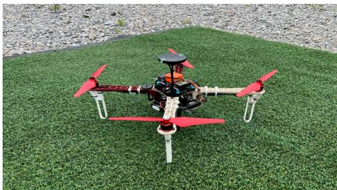
Fig. 3. Drones built with the Pixhawk system
