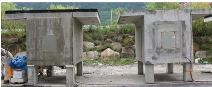
Fig. 1. Bridge specimens of first year
