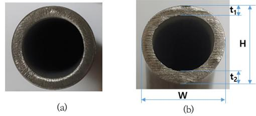
Fig. 3. Cross-section of the hydraulic tube
