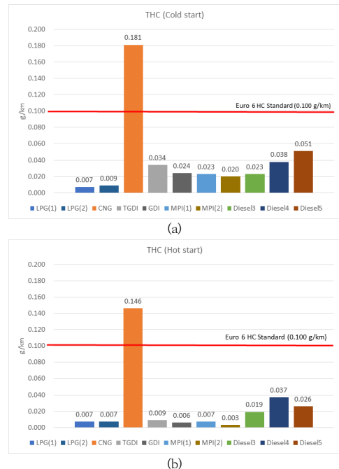
Fig. 2. THC emissions according to vehicle type under (a) cold-start and (b) hot-start conditions
