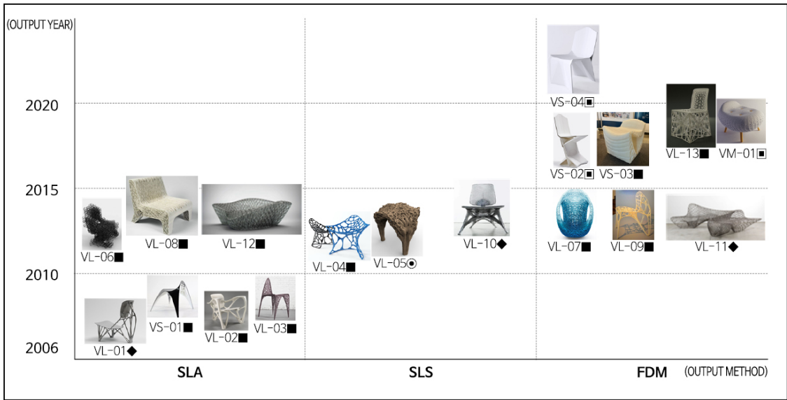
Line(VL), Surface(VS), Mass(VM), Plastic(■), Reusable/Eco-friendly plastic(□), Metal(◆), Cement(●), Food ingredients(◎), Wood(▲) Fig. 1. Voronoi design according to 3D printing output method by year
