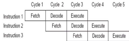
Fig. 1. Three stage pipeline of Cortex-M4
