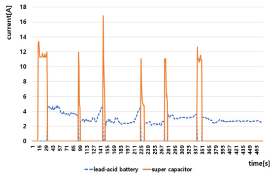
Fig. 12. Current characteristics of hybrid electric wheelchair
