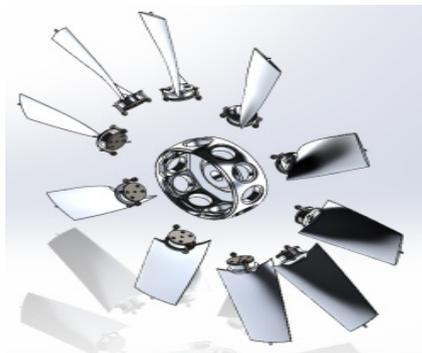
Fig. 4. 3D Model exploded view for Axial fan for ventilation smoke
