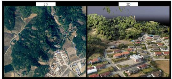
Fig. 9. Comparison between conventional methods (aerial photography) and 3D survey methods (obstacles)
