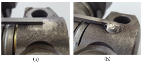
Fig. 3. Before and after for spot on top of cap (a) Before spot welding (b) After spot welding
