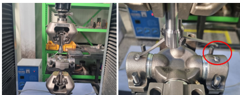
Fig. 12. Wire welding strength confirmation test
