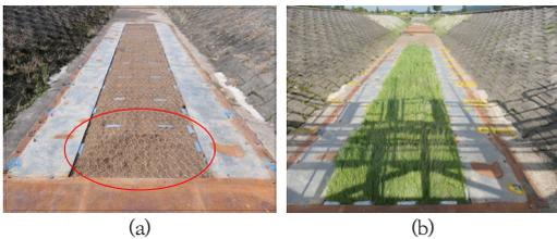
Fig. 12. Appearance of the non-vegetated (a) and vegetated (b) specimens after the 3rd run of the each experiment.
