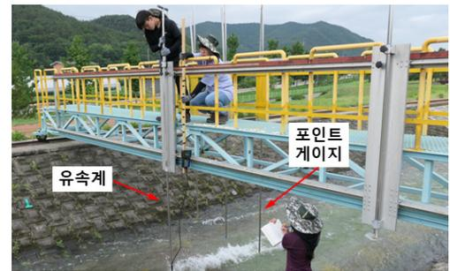
Fig. 6. A picture of hydraulic measurements
