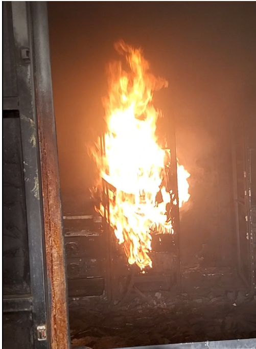
Fig. 10. Top fire stage of 25kWh Rack
