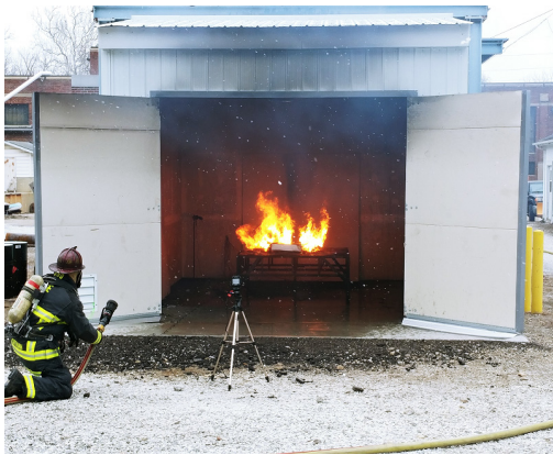
Fig. 18. Battery module thermal runaway and fire test
