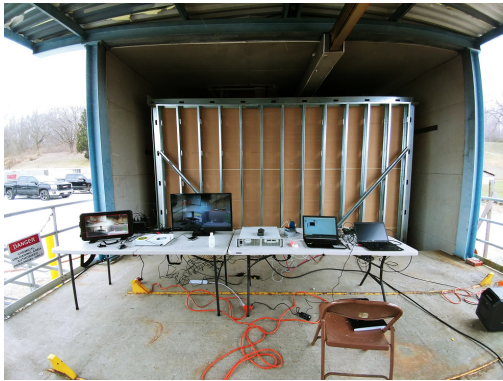
Fig. 17. Fire detection and prevention demonstration facility for battery module based on gas detection
