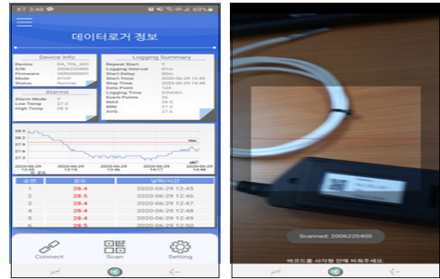
Fig. 13. Data Logger Display and QR-code scanning function
