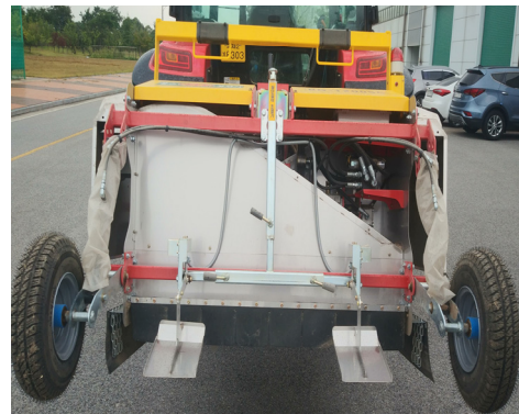
Fig. 4. Configuration diagram of the onion stem cutting prototype attached to tractor.
