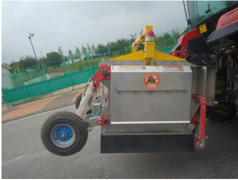
Fig. 5. Photograph of the onion stem cutter attached to tractor.
