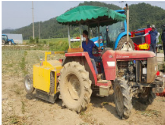
Fig. 3. View of the onion cutting prototype attached to tractor.
