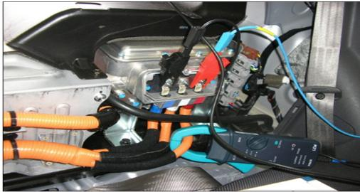
Fig. 7. Insulation Measurement of Safety Plug Terminal Using Insulation Measuring Instrument.
