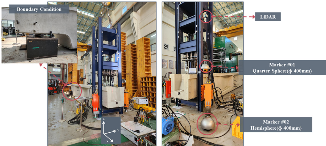
Fig. 7. Test setup for verification of relative position estimation method on remote precision installation robot prototype
