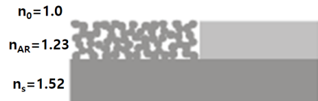
(a) \lambda/4 single layer AR coating (porous structure)
