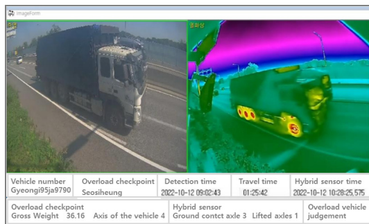
Fig. 11. Checking the case of an overloaded vehicle through variable axis operation during performance evaluation
