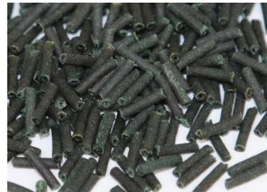
Fig. 3. Shape of sample(single perforated propellants)
