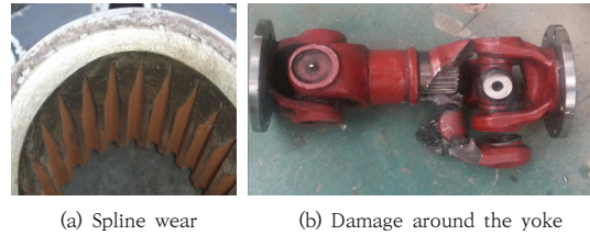
Fig. 2. Cradan shaft failure type
