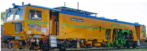
Fig. 1. Work by switch tie tamper
