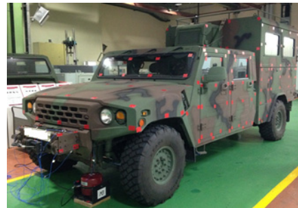
Fig. 5. The figure of accelerometer setup for modal test
