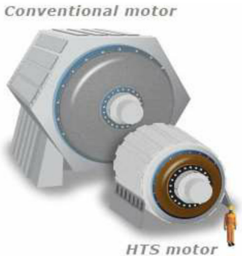
Fig. 5. Size of traditional motor and HTS motor
