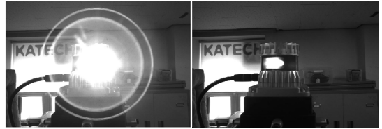
Fig. 9. LiDAR picture with a near-infrared camera when the synchronization board is operating
