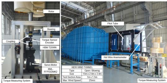
Fig. 10. Open-jet type wind tunnel facility and experimental setup
