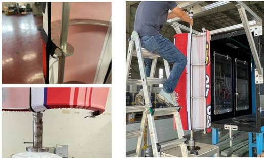
Fig. 9. Proto-type Fabric rotor(Savonius type)
