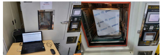
Fig. 8. Low temperature storage test environment
