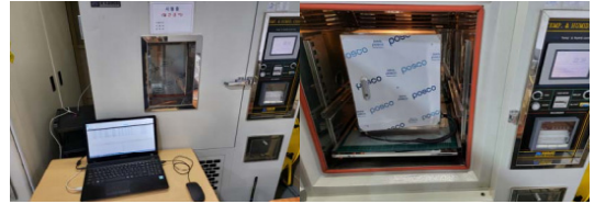
Fig. 6. High temperature storage test environment
