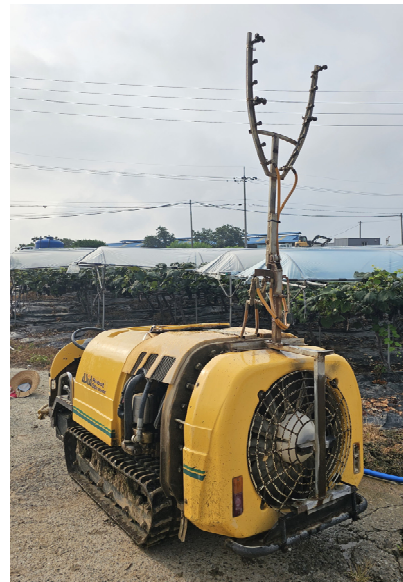
Fig. 2. Y-type spray nozzle installed on Speed sprayer.
