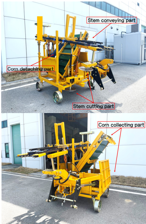
Fig. 2. A photo of fresh corn harvester for agricultural tractor with major components
